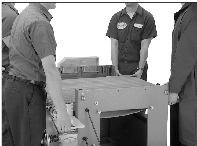
Figure 50. Lifting the table off of the drum sander cabinet with four people.
